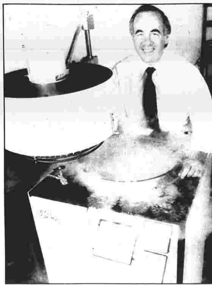
DEEP FREEZE — Bruce Norian, co-founder of Applied Cryogenics Inc. in Newton, Mass., shows off one of the company's deep freezers. The 2-year-old company hardens industrial tools to lengthen their lives, and experimenting has also produced golf balls that fly farther and violin strings that stay in tune longer.
